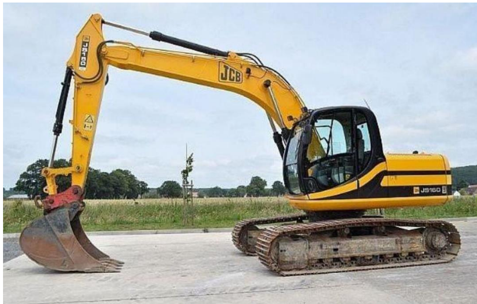
Photo 1 - Tracked excavator with bucket for excavation
