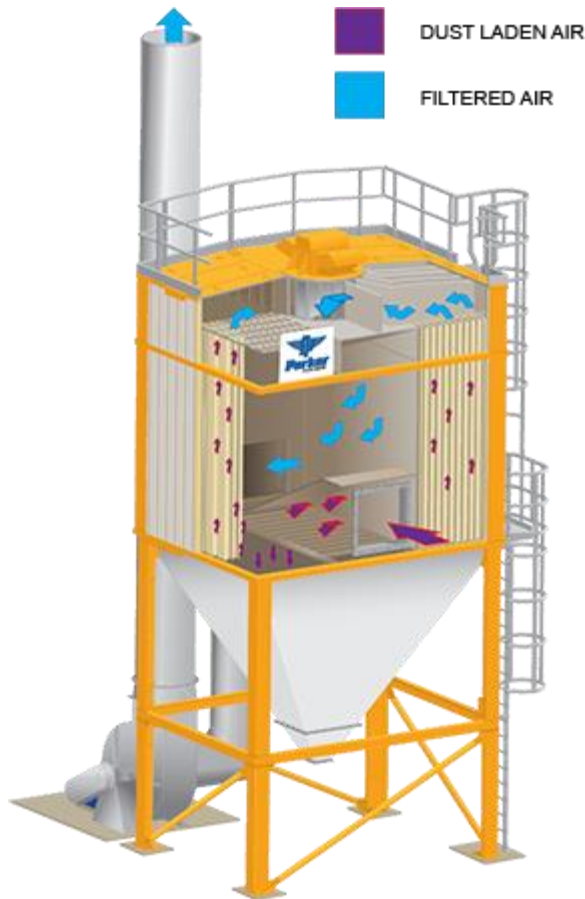
Figure 4-4: Secondary dust collection system (bag filter)
