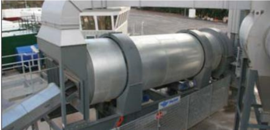
Photograph 4-3: Typical aggregate dryer
