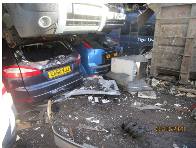
Figure 5. Ford focus (NJ57 XYX) stored with visible oil contamination indicating a leak from the vehicle stored above
