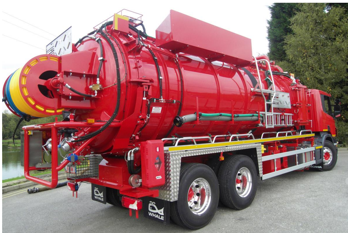
Typical high pressure jet vac lorry
