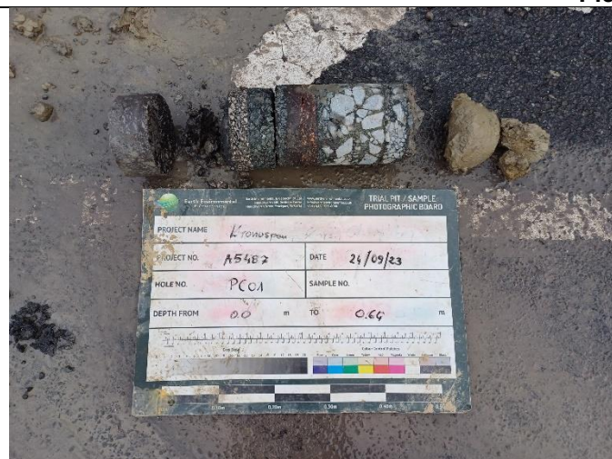
Pavement Core 01: Concrete core sample
