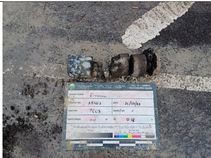
Pavement Core 03: Concrete core sample
