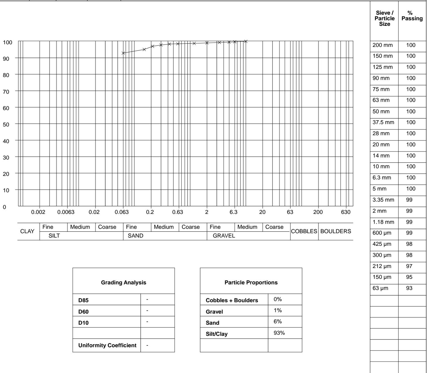
**Method of Preparation** : BS 1377:PART 1:1990:7.3 Initial preparation 7.4.5 Particle size tests
