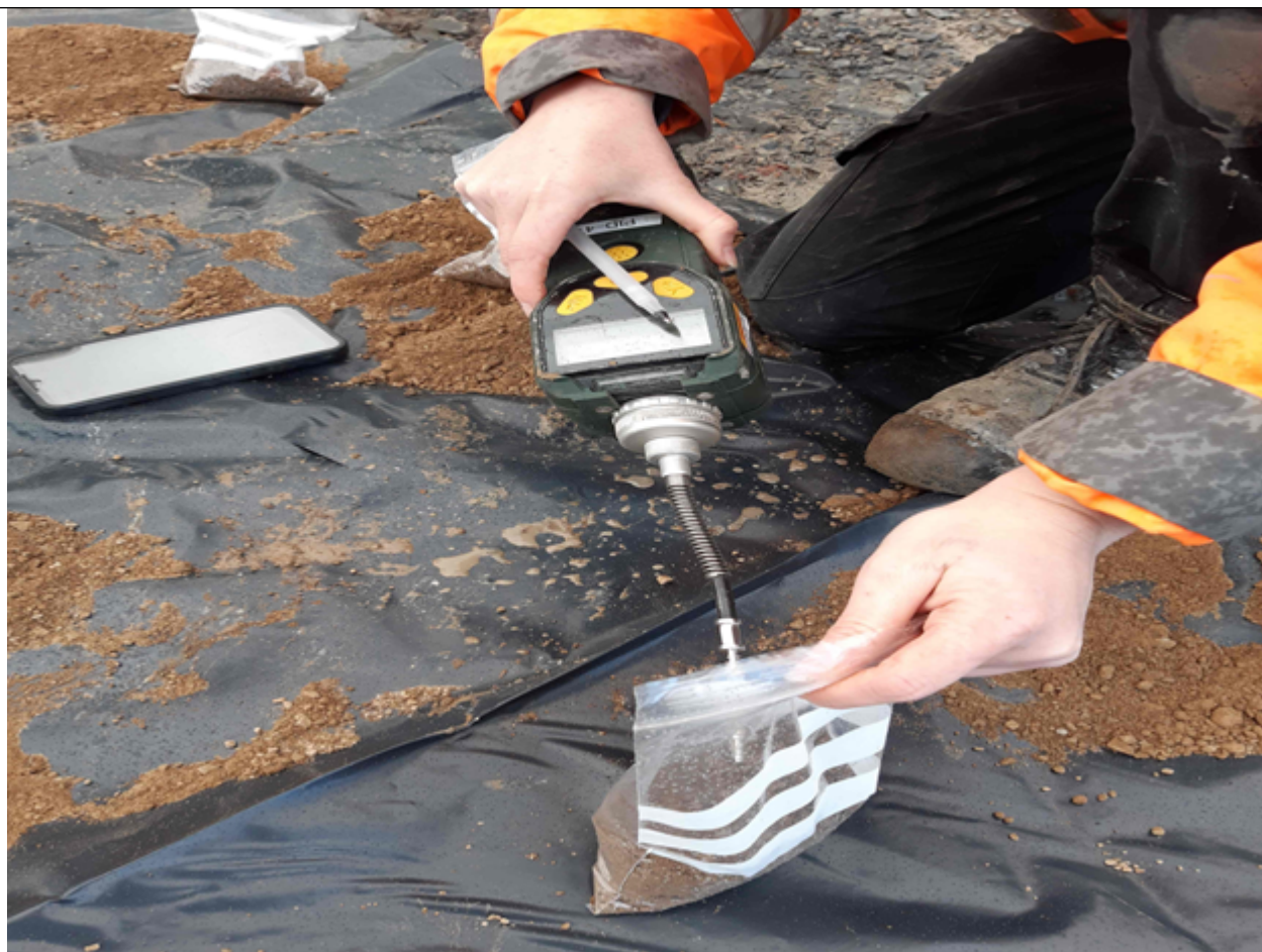
Photo showing sample being tested for VOCs
