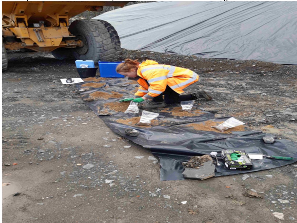
Photo showing sampling of sieved soil
