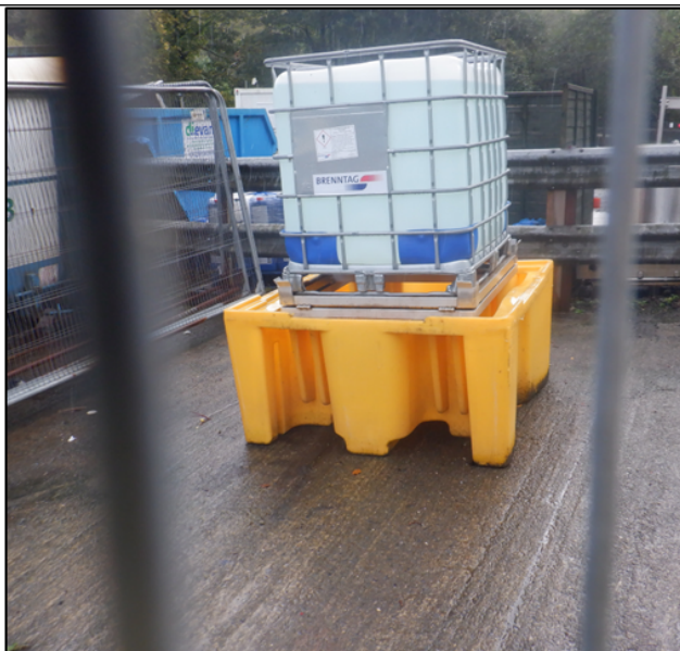
Image 2 – showing an IBC storing calcium chloride with secondary containment, taken at 11:01 on 19 October 2023
