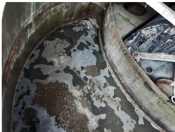
Figure 2: Primary chamber of treatment system
