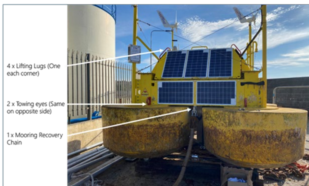
Figure 16: FLS200 buoy lifting points.
