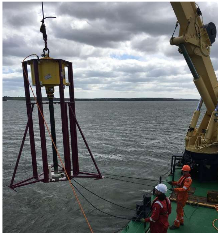
Figure 8. Deployment of Vibrocorer from Survey Vessel.
