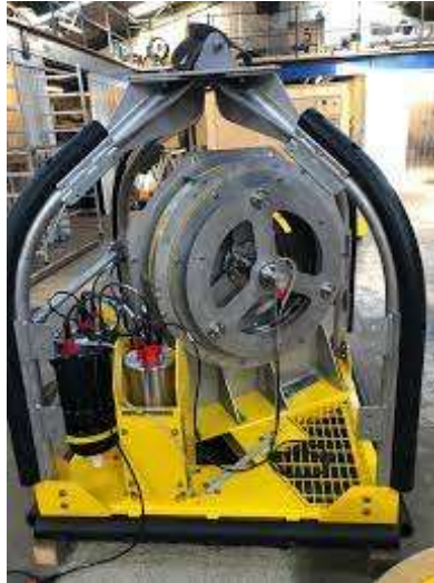
Figure 7. Neptune 3000 CPT rig.
