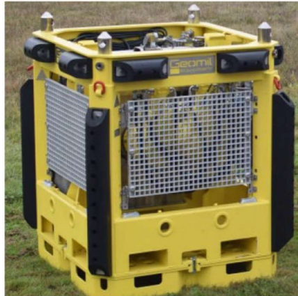
Figure 6. Geomil Manta 100DW CPT rig.
