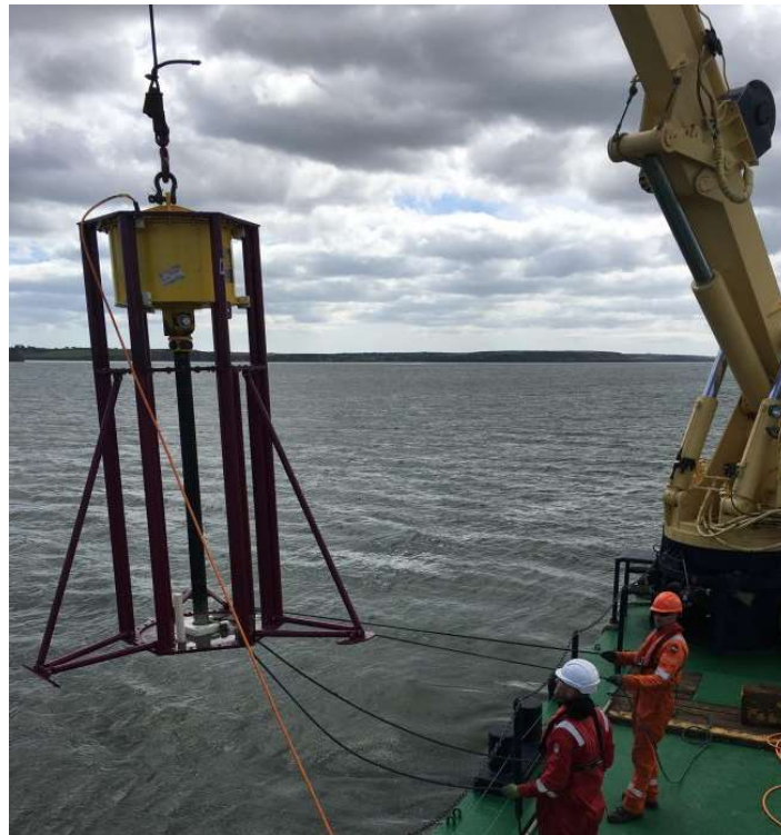
Figure 8. Deployment of Vibrocorer from Survey Vessel.
