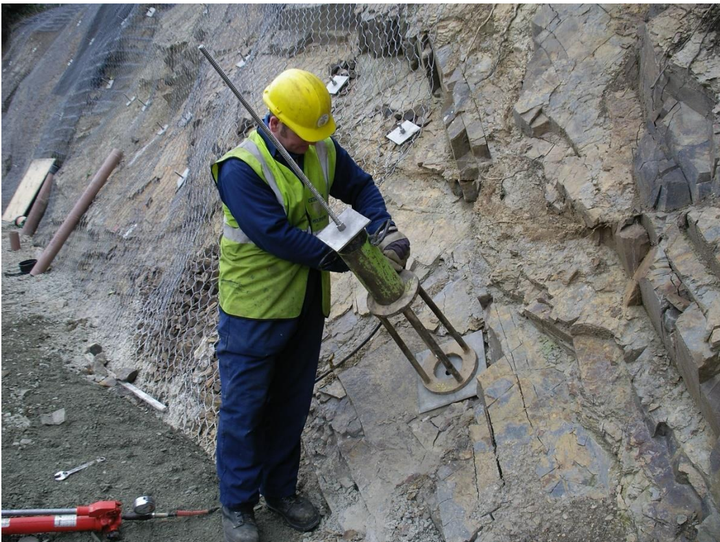
Photo 2 Connecting to hand pump.
