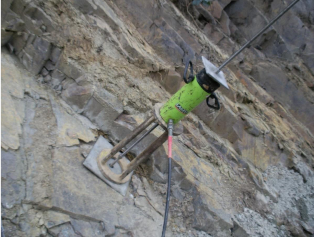
Photo 1 Typical setup for testing (Reaction plate, articulation stool and stressing jack)
