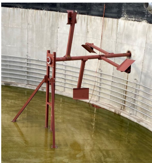
Figures 2 and 3. Photographs showing paddle stirrer (left) and submersible stirrer (above).
