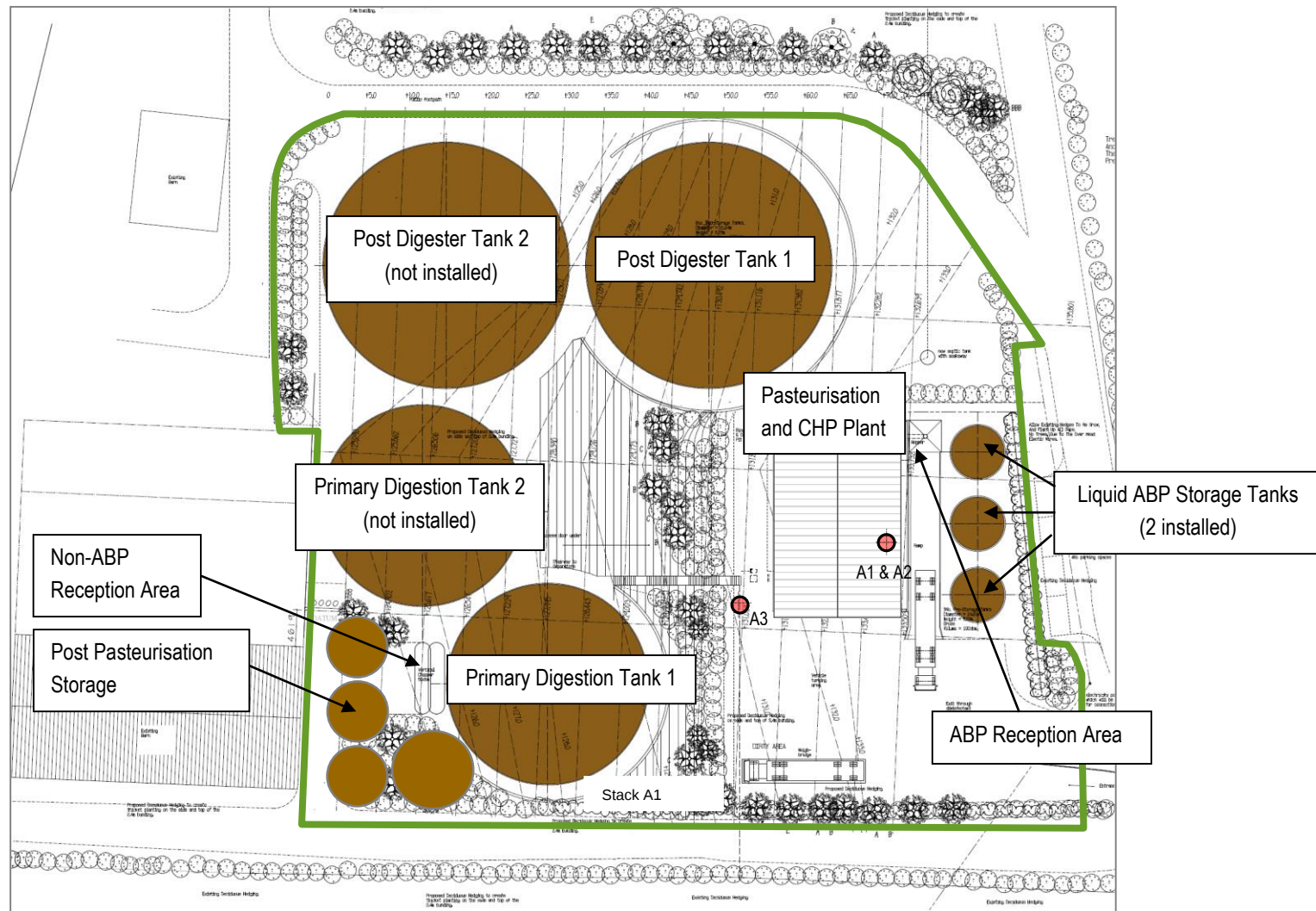
Figure 1.2: Installation Boundary and Plant Layout
