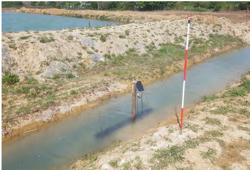
Figure 7: In-situ turbidity measuring device used by frog environmental.
