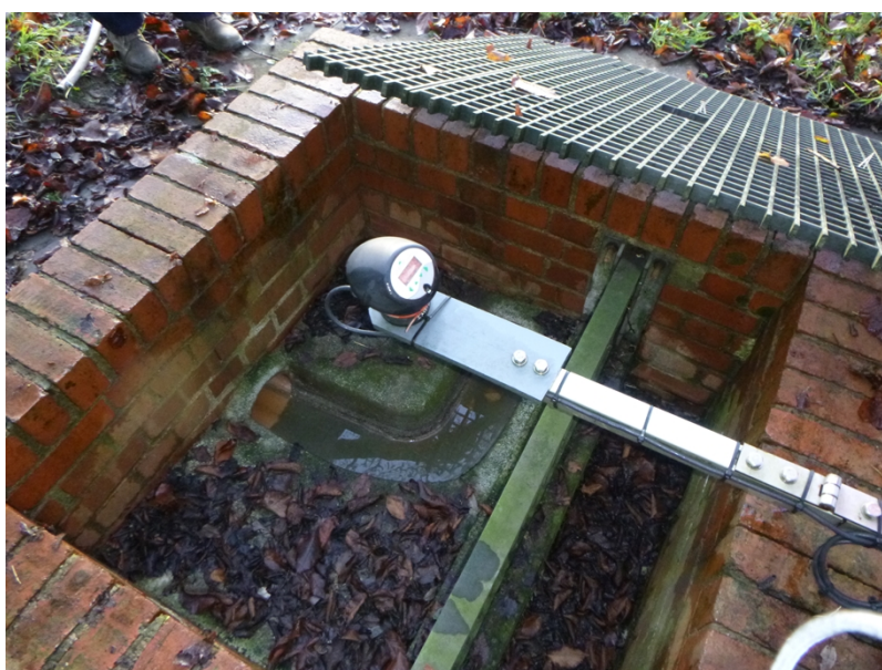
Photograph 3: EDM recorder above Clarach STW inlet
