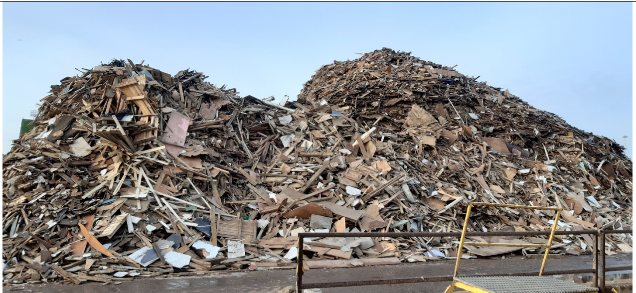
Photo 2 - Large stockpile of unprocessed wood not in compliance with the sites FPMP
