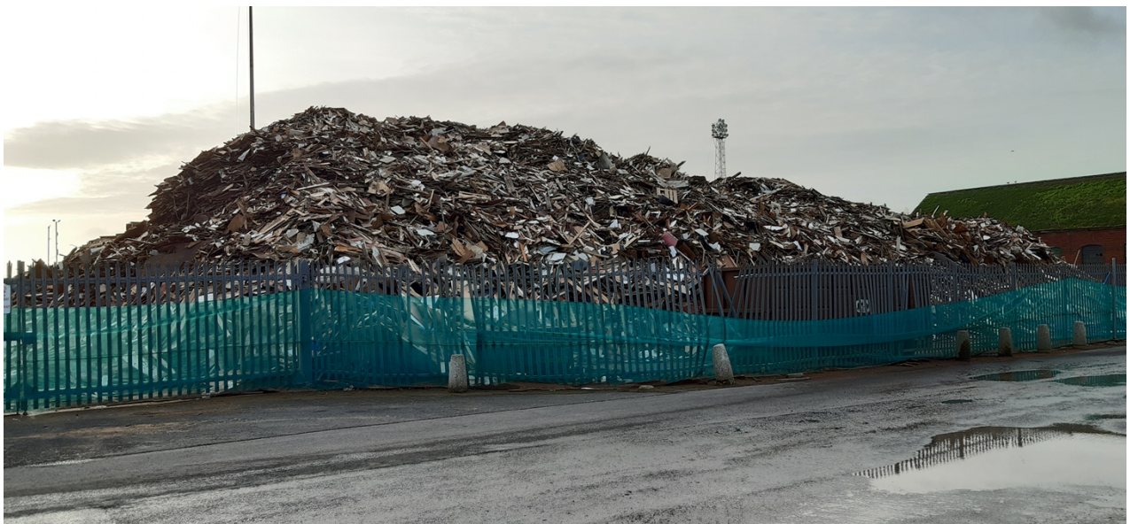
Photo 3 - Large stockpile of unprocessed wood not in compliance with the sites FPMP
