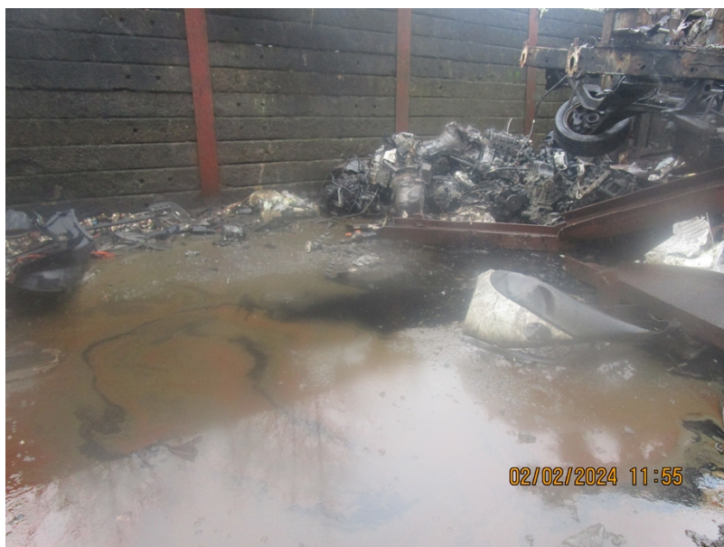
photo 2 pooling of contaminated water
