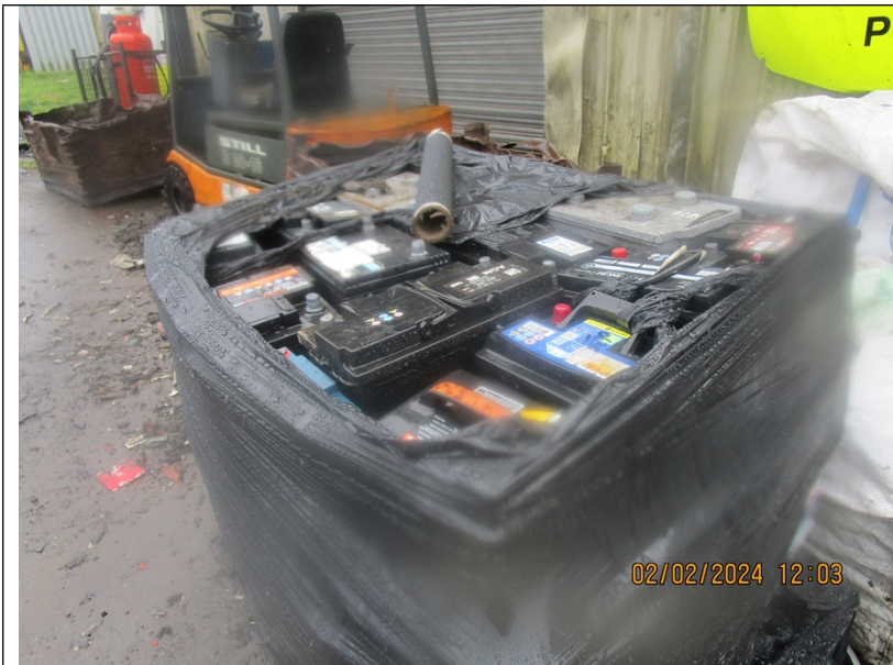
photo 4 batteries being stored outside with no lid
