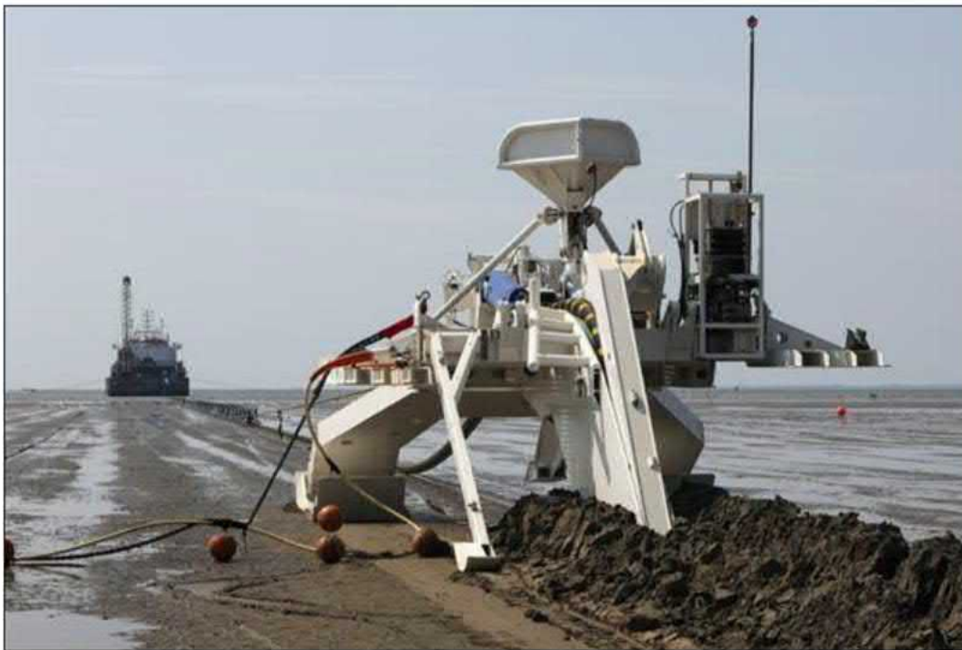
Photograph 2: Typical cable plough (Photo Credit Boskalis)
