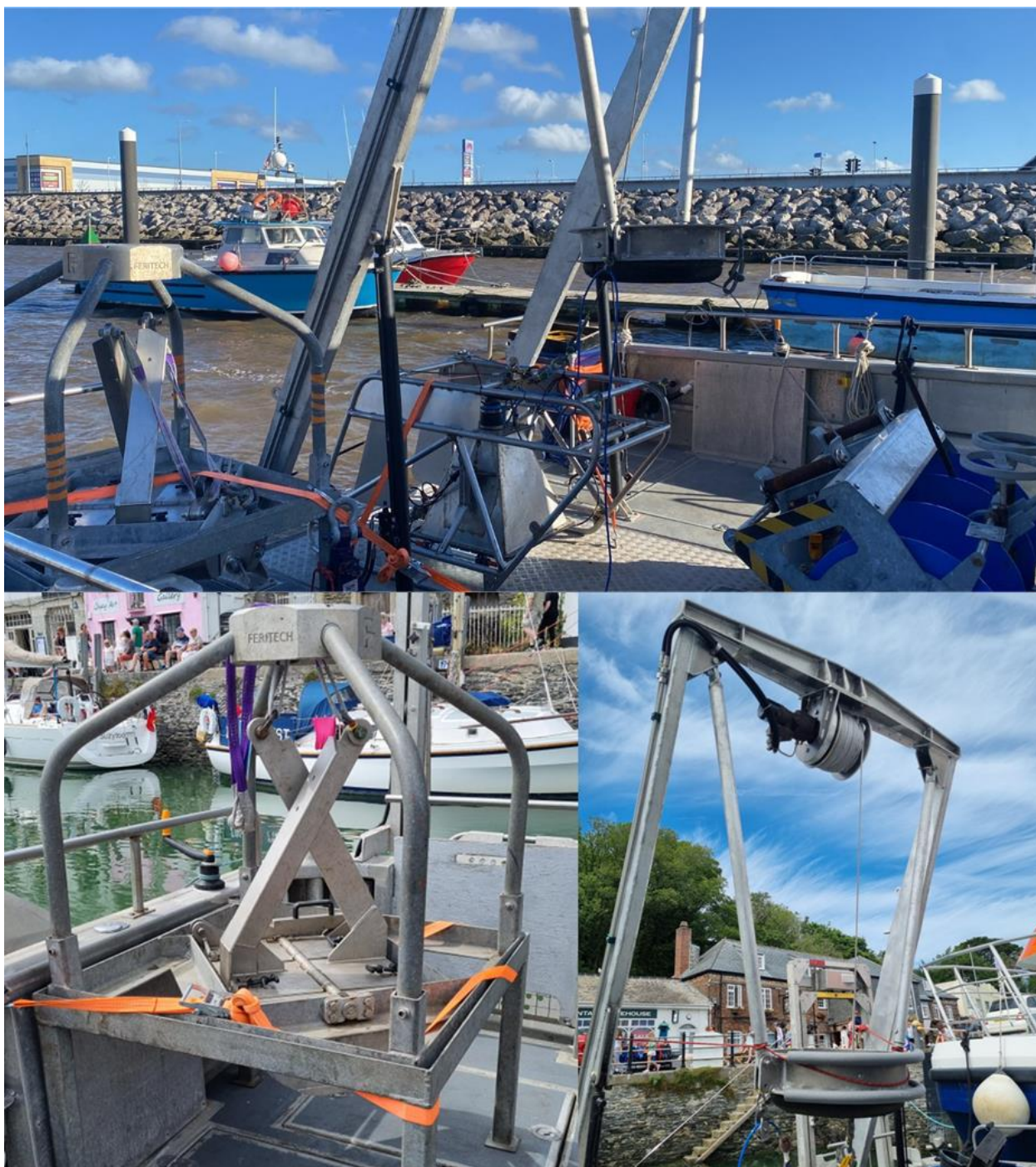
Plate 2 DDC system (top), DVV grab (bottom left), and equipment dampener (bottom right) mobilised aboard the Argyll Explorer.
