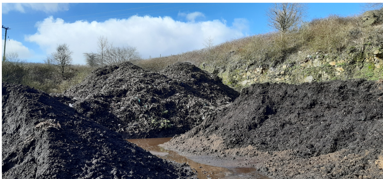
Photo 14 - Stockpiles of unprocessed green waste (background) in composting station area not in compliance with sites FPMP document
