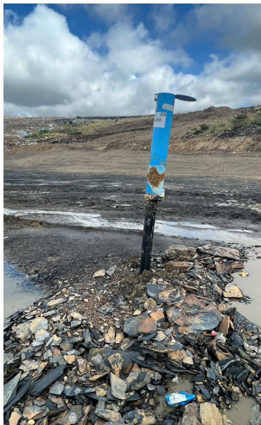
Plate 4-1 Wellscreen After Ground Level Reduction
