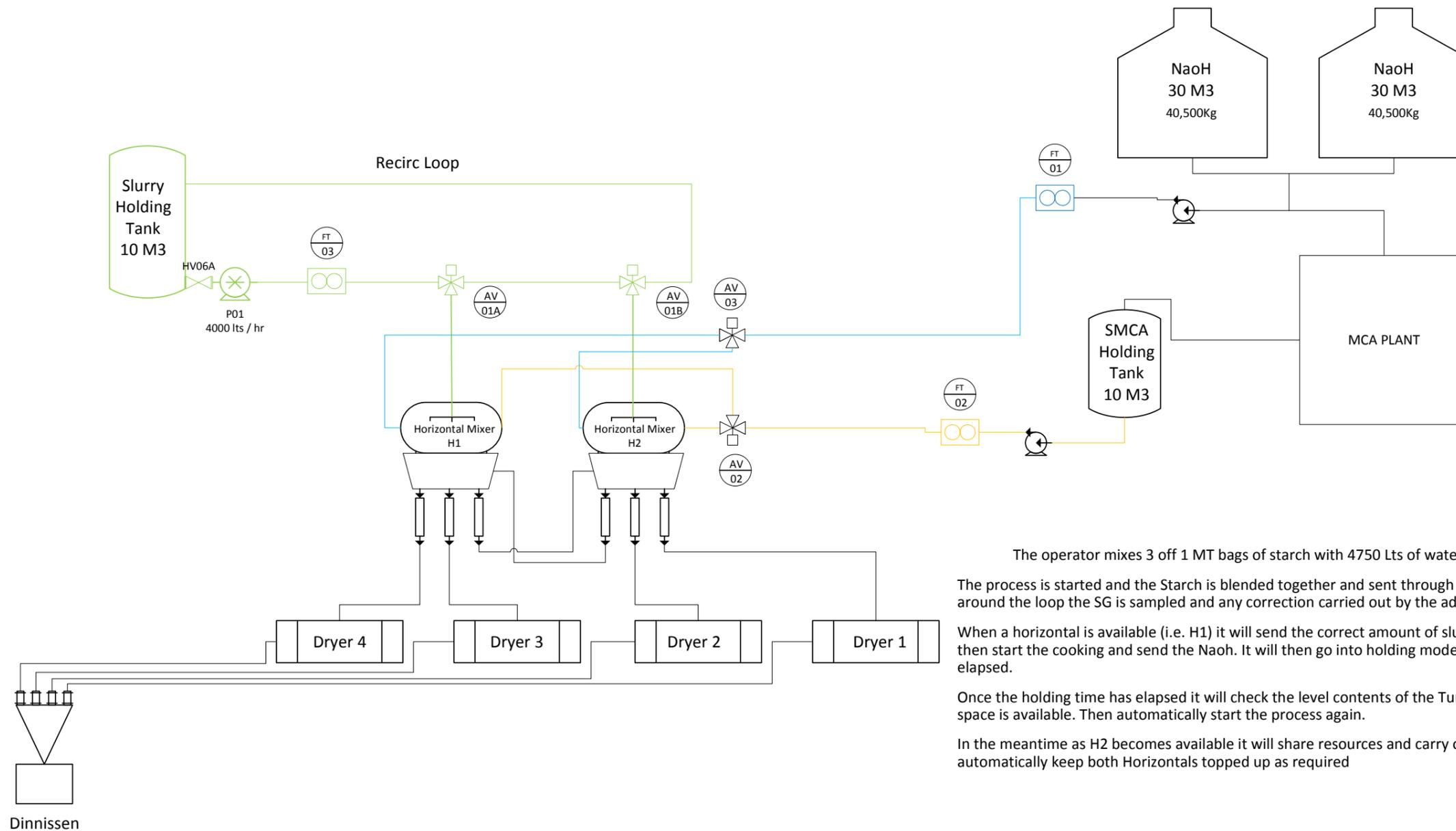
The operator mixes 3 off 1 MT bags of starch with 4750 Lts of water and adds the crosslinker
