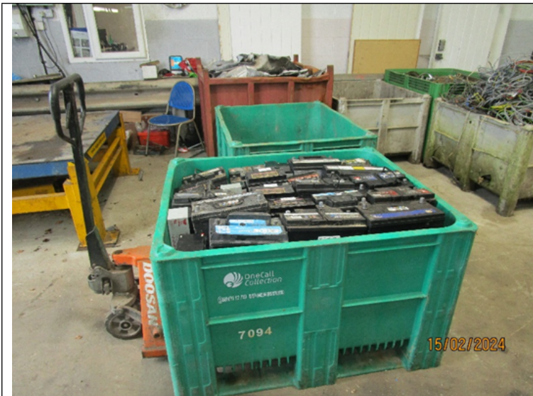
Figure 1. Segregated and sorted waste metals and waste batteries stored in bins inside site working shed.
