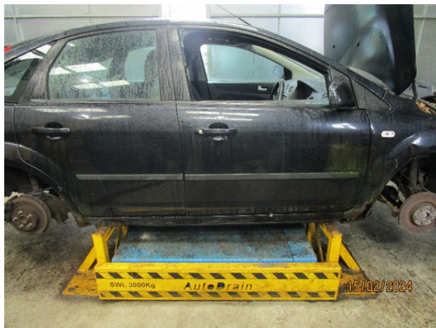
Figure 2. depolluted ELV inside depollution shed.
