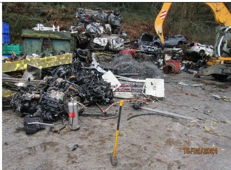
Figure 3. Crushed depolluted ELV's stored outside on impermeable surface.
