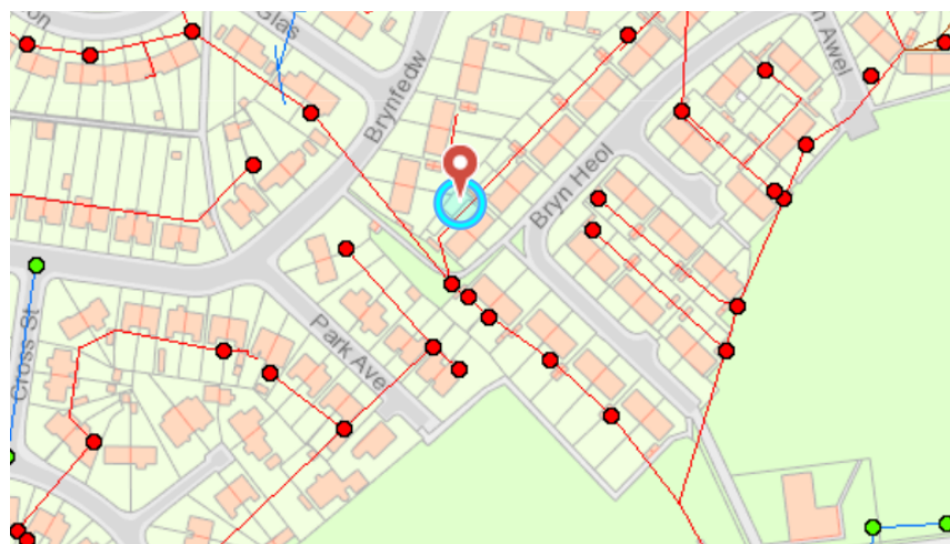
Fig 1. Surface water discharge point
