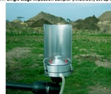
Photograph 5.1: Single stage impaction sampler (Andersen) set up in the field
