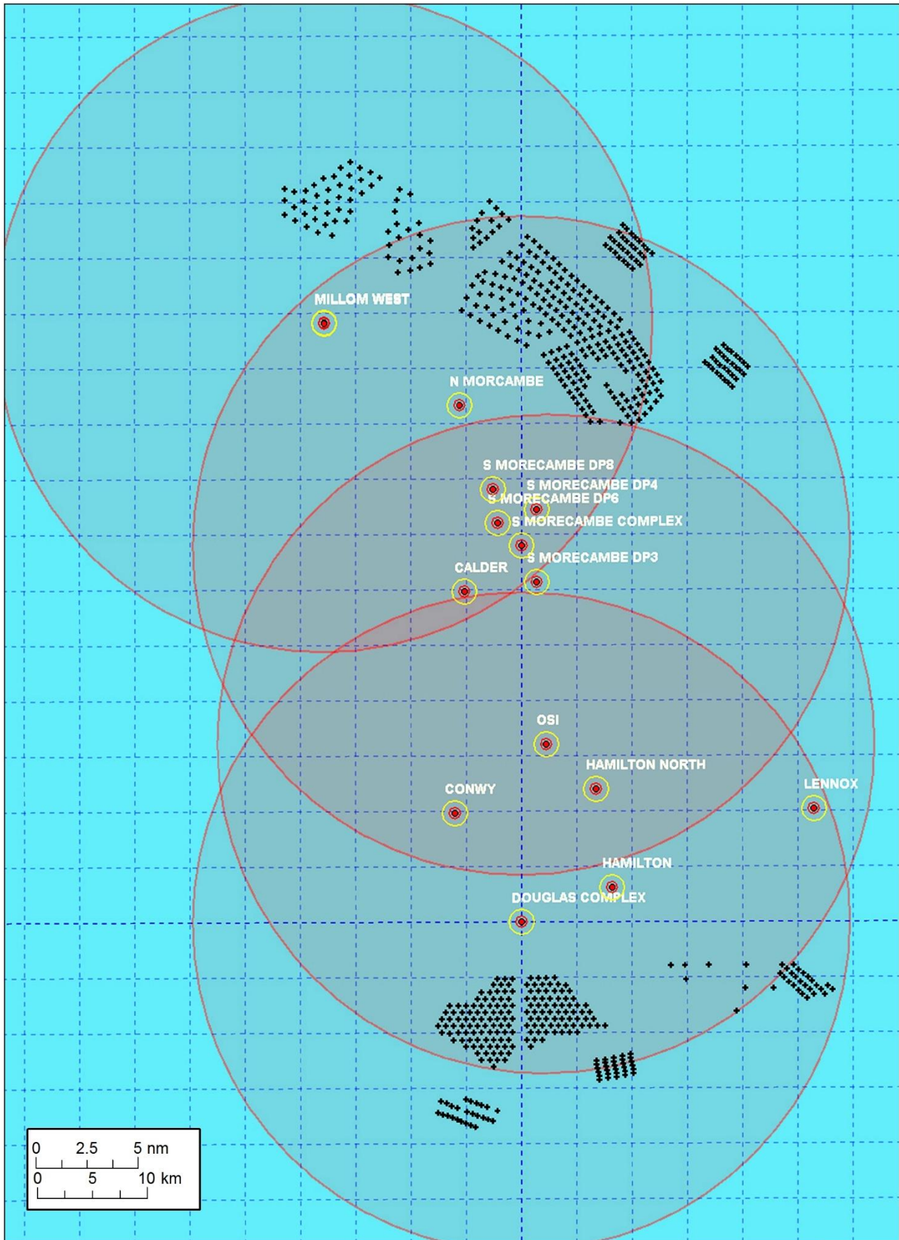
Figure 1.11: Modelled layout of the base case scenario showing the location of the existing wind farms and the coverage of the REWS in the region.
