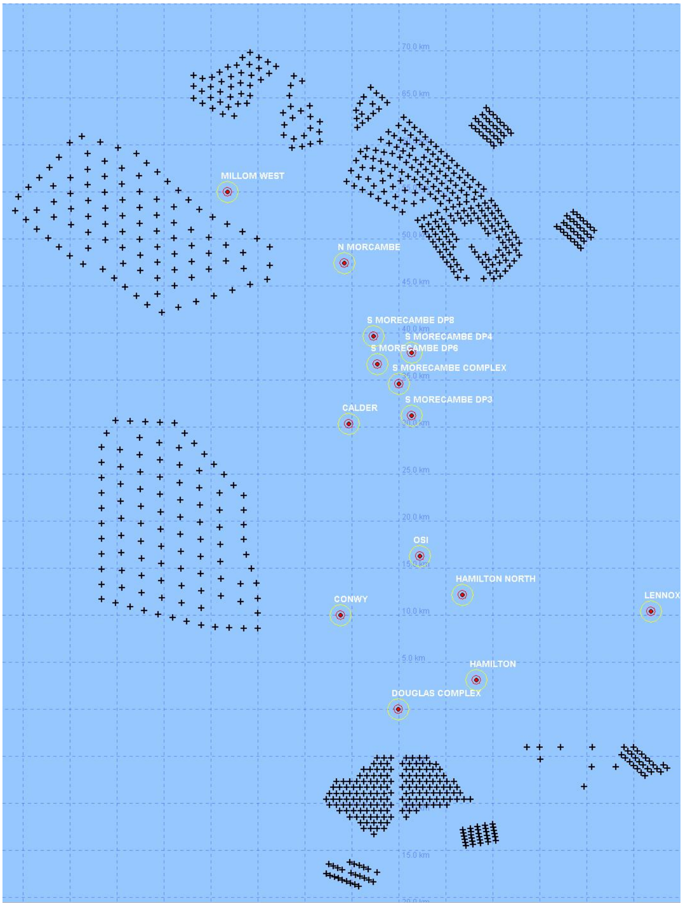
Figure 1.40: Modelled cumulative layout of the Mona Offshore Wind Project and Morgan Generation Assets showing the indicative location of the wind turbines and the location of oil and gas platforms in the region.
