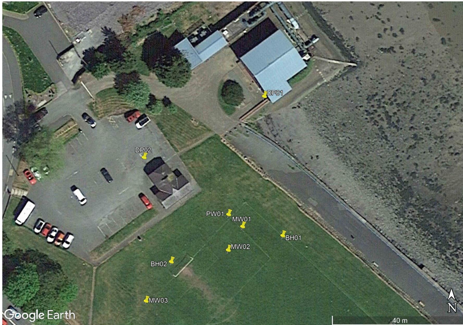
Figure 1: Indicative Pumping Test Layout.
