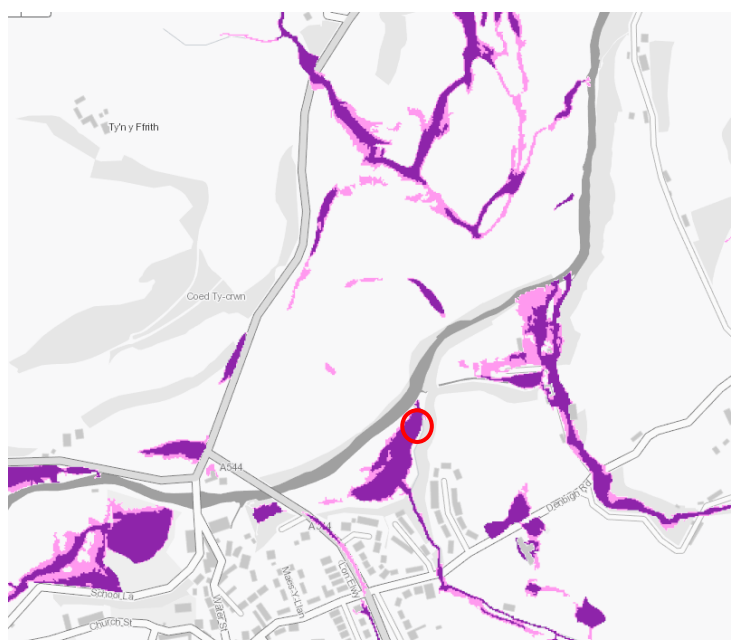
Figure 4: Surface water and small watercourse flood extents around the weir (circled in red) extracted from NRW mapping [1]
