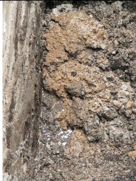
TP101 – Water strike from saturated soils
