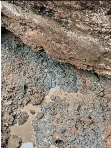
TP104 – Water strike in sand/gravel
