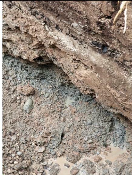
TP104 – Side wall collapse due to running sands
