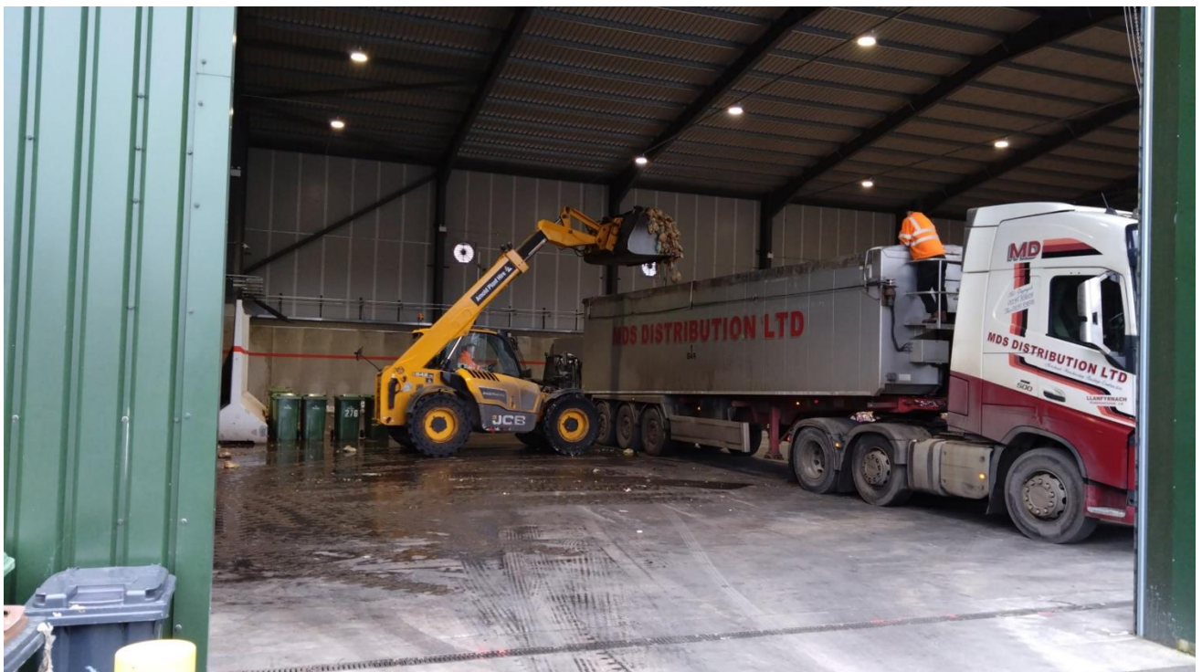
Figure 3-3 – Telehandler loading a bulk lorry with food waste in the shed
