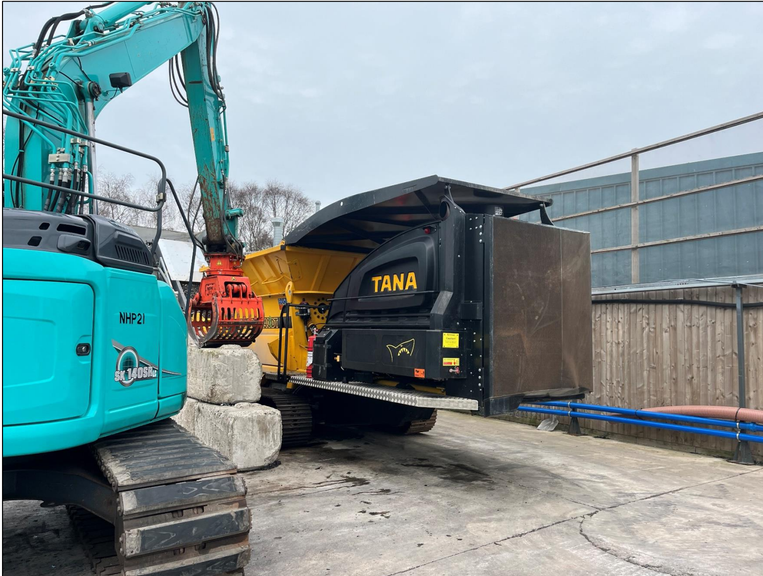
Figure 8: Photograph of the existing Tana Shark Shredder 440 DT at Unit 27. This must only be used for transporting and must not be used for shredding
