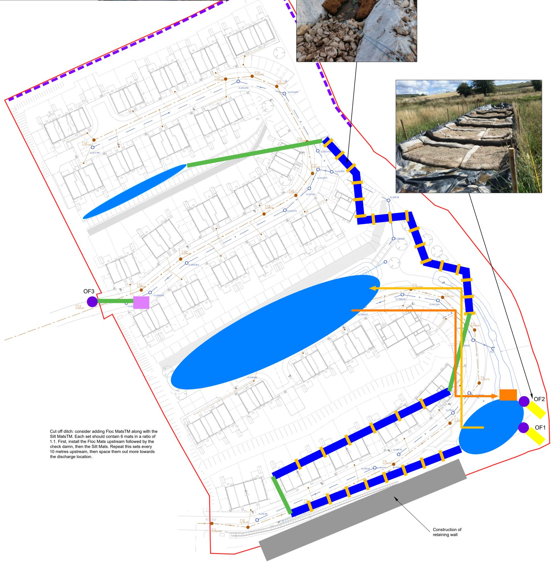
Cut off ditch: consider adding Floc Mats™ along with the Silt Mats™. Each set should contain 6 mats in a ratio of 1:1. First, install the Floc Mats upstream followed by the check dam, then the Silt Mats. Repeat this sets every 10 metres upstream, then space them out more towards the discharge location.
