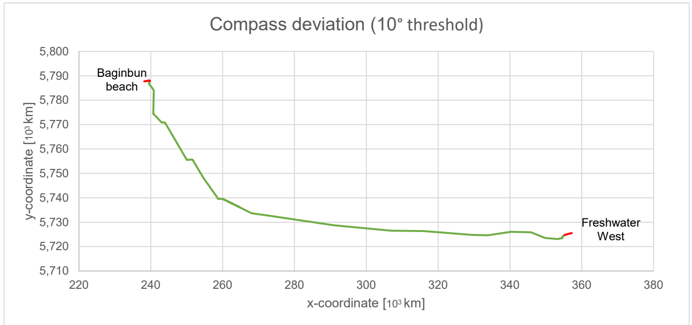
Figure 4.2-9: Calculated compass deviation along the Greenlink offshore cable route with 10° angle threshold.
