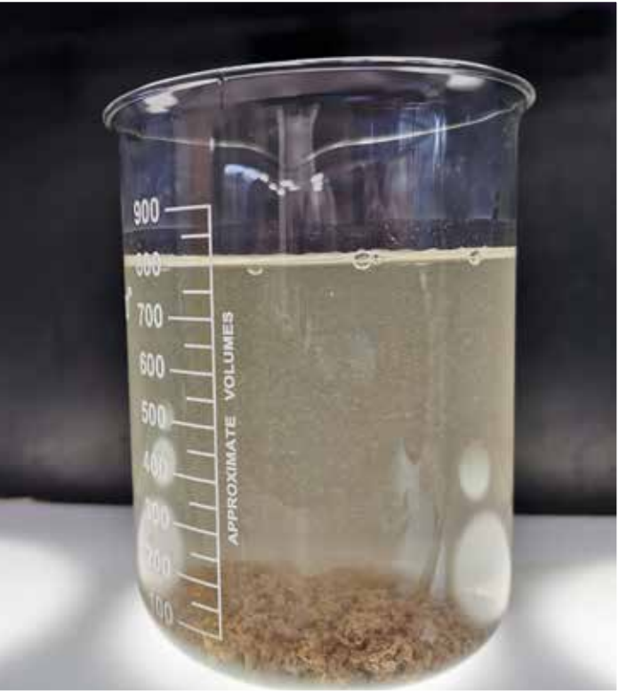
Clay flocs rapidly formed after chemical dosing
