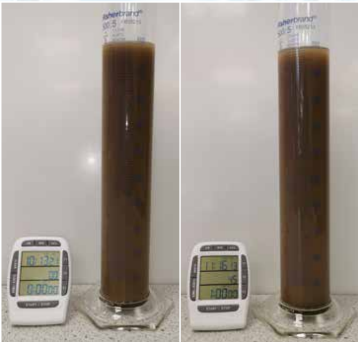
Settlement of clay particles from time 0-60 mins
