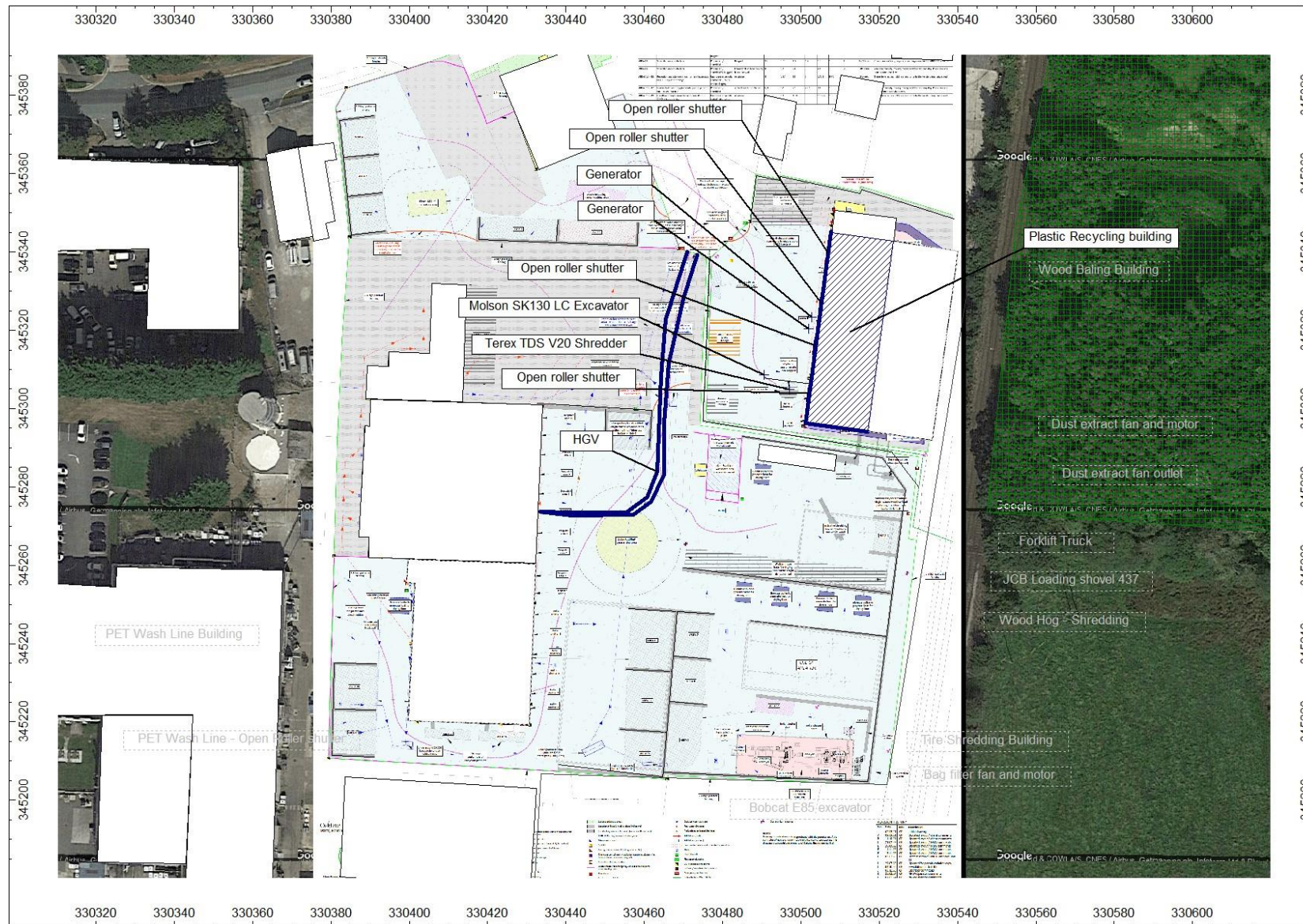
Figure C1: Site plan indicating grid coordinate references x, y coordinates for all external modelled noise sources (existing site)
