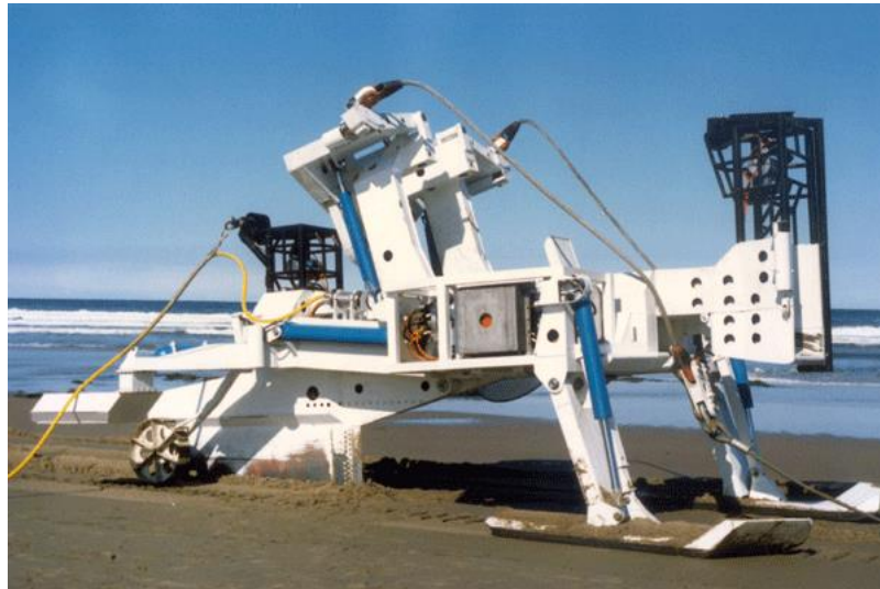
Figure 4-23. Illustration of a typical cable plough (KIS-ORCA, 2024)
