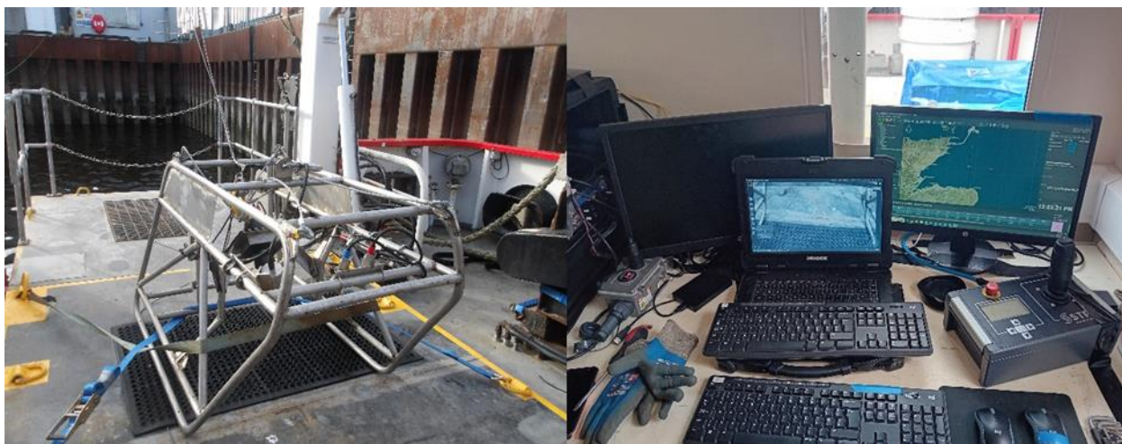
Plate 2 Left: OEL CLOC camera system. Right: The camera system topside setup.
