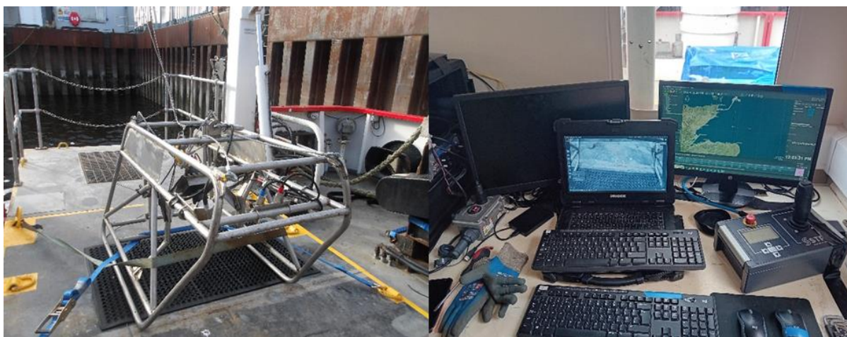
Plate 2 Left: OEL CLOC camera system. Right: The camera system topside setup.
