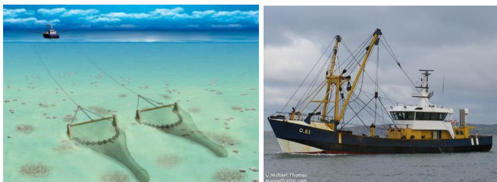
Figure 26.1-15: Typical beam trawler and gear diagram (Source: Seafish, 2015; MarineTraffic, 2022)
