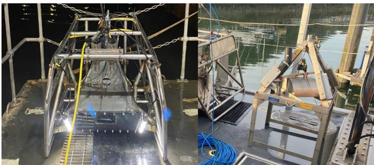
Plate 2 Left: OEL's freshwater housing camera system. Right: 0.2 m 2 Day Grab
