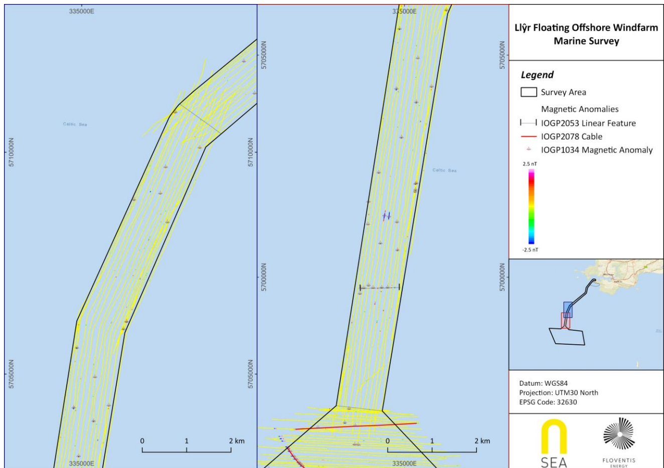
Figure 5-48: Overview of magnetic survey results – ECR South
