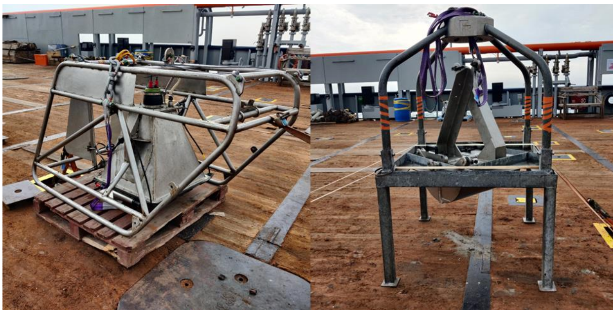
Plate 2 Left: OEL's freshwater housing camera system. Right: 0.2 m 2 DVV Grab.
