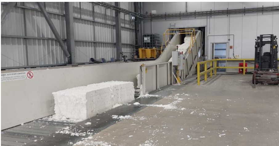
Photograph 1-5: Broke conveyor
