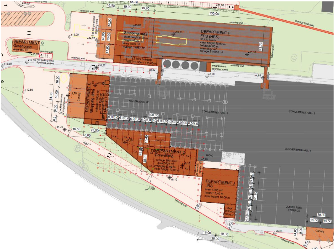
Figure 6 - West end development showing reel store ("J"), converting and shipping and high-bay warehouse ("F").
