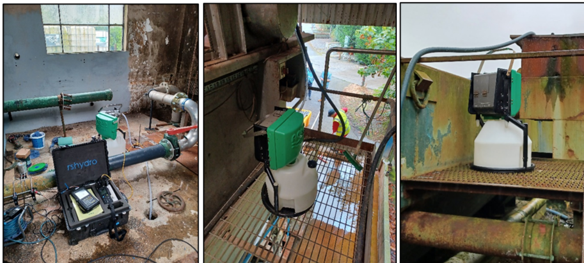
Image 1: Autosamplers fitted pre-treatment (left), during treatment (mid) and post-treatment (right)
