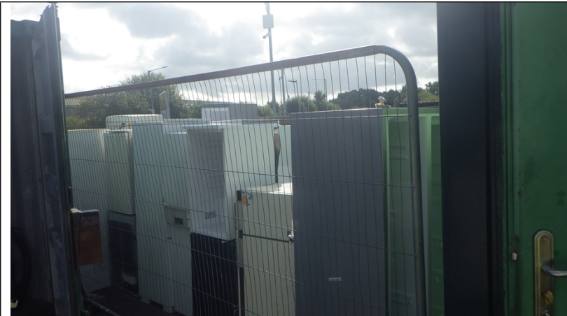
Photograph of Fridge/freezers without weatherproof covering and sealed drainage.
