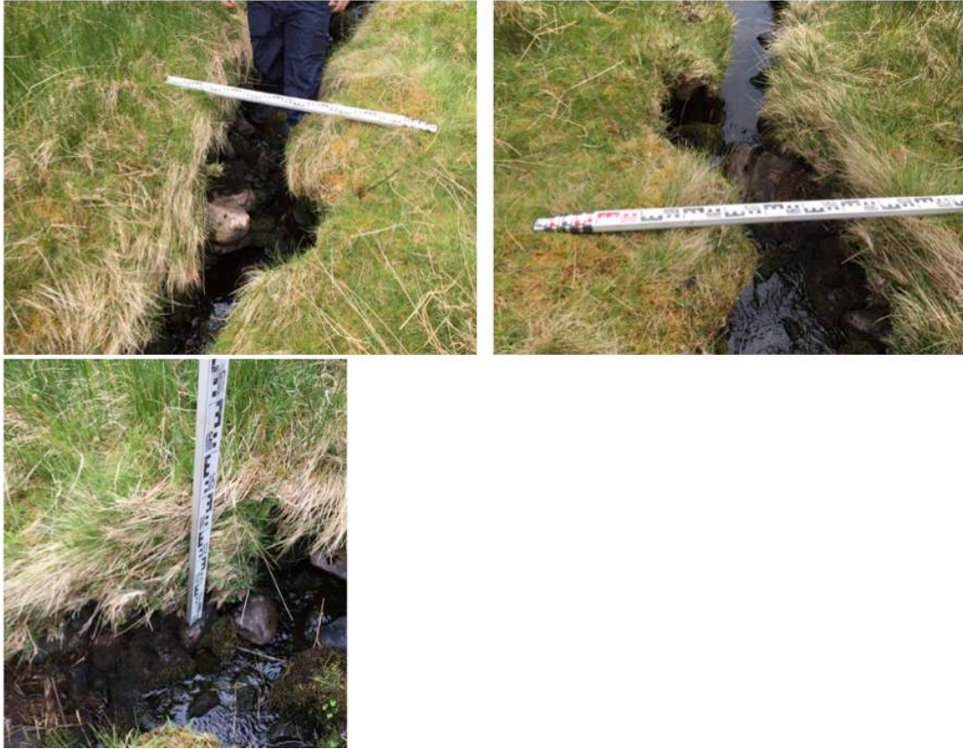
Fig 11 (u/s), 12 (d/s) & 13 (close up of watercourse bed): Feeding Intake location, 500mm wide channel, watercourse is dominated by bedrock overlaid with small gravels, both banks are well vegetated promoting a stable environment (SN 76628 22209).
